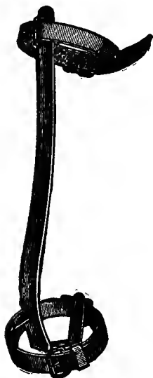
FIG. 228.—Eastern pole climbers, with and without strap for attaching to legs.
